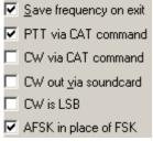
and neither the CAT nor any of the Com Port configuration settings should have CW via DTR or CW via RTS selected.
