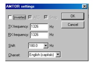
The TX and RX frequencies show the position of your cursor is in the spectrum window. Keeping this around 1500 Hz, will keep your transceiver operating close to the center of its pass band. Shift is selectable (if you don't see what you want in the drop down box, any number can be typed in). Most AMTOR uses a shift of 170 Hz. You can invert the Mark and Space signals by checking the "Inverted" box.
